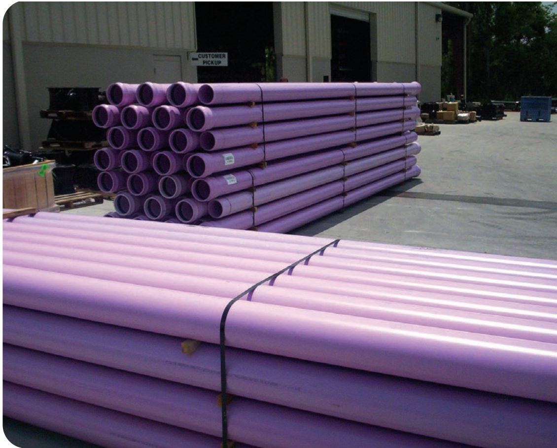
Reclaimed water pipe
